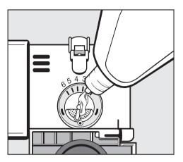
Add rinse aid only until it is visible on the surface of the filter in the opening.
